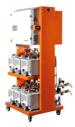
The **integrat 80** is used for the modular temperature control with water up to 140°C in the basic version with up to six temperature control circuits to be operated completely independently of each other. The basic version can be expanded with extension columns and up to 24 temperature control modules.
